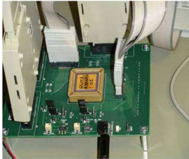
Caption: Test board and ASIC incorporating a double-memory programmable and configurable PWAG controller
